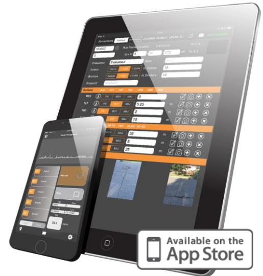
Mobile devices apps, iPhone rRuf and iPad rInspector , are used to collect roughness and pavement distresses respectively.
